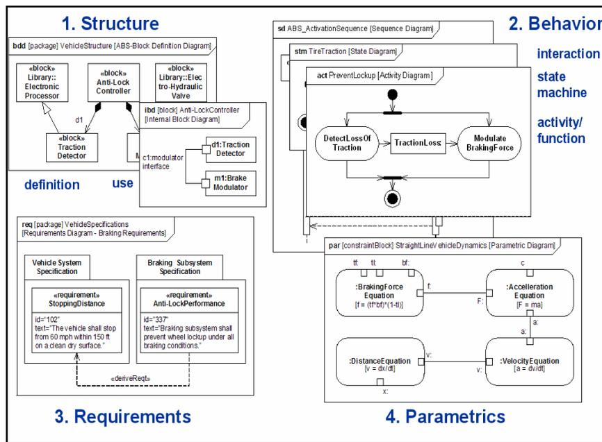
Figure 4: The Four Pillars of OMG SysML
