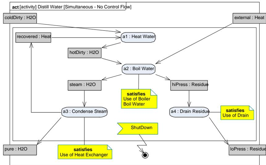
**Figure 6: Distil Water Activity with Requirements**
