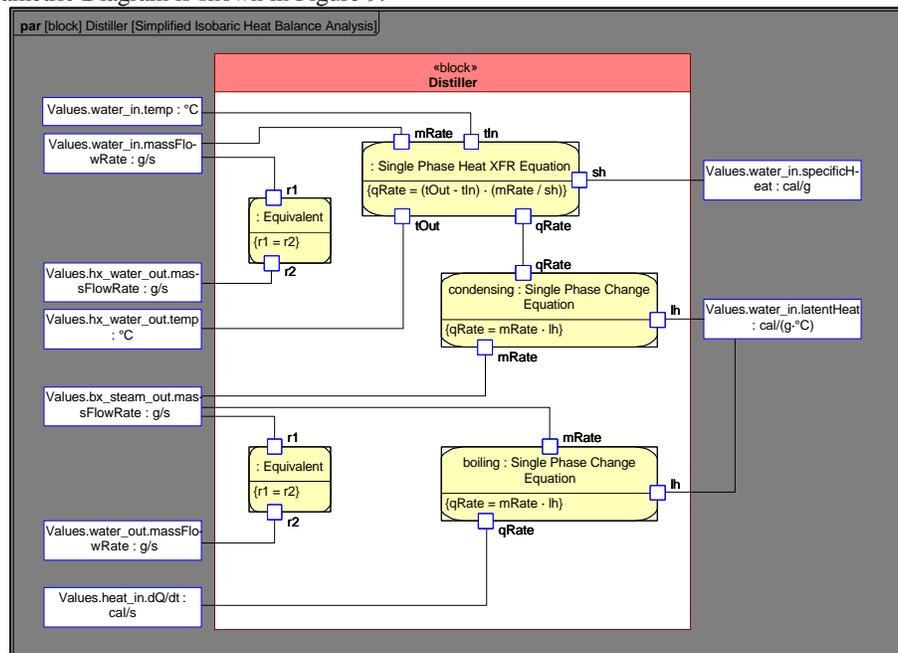
Figure 9: Parametric Diagram
