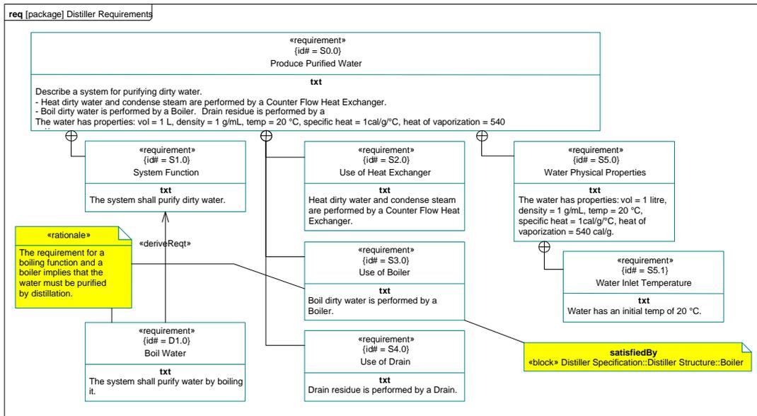
**Figure 5: Requirements Diagram**
